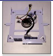
Connect the Smart-Connect base wiring to the light circuit wiring of the building.
