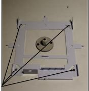
2. Mount Smart-Connect base by fixing it to the ceiling at all four corners. Minimum size fixing: 6.5mm. If fixing to plasterboard use 4 hollow wall anchors.
