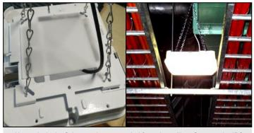
5. Alternatively the fitting can be suspended from the ceiling. Connect the IP65 plug to the fitting then attach the chain to the base plate (as shown above) and wire the mains cable into a junction box.
