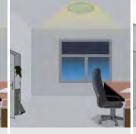
After the hold time the light switches to standby mode. If twilight time is set to *infinity* the light remains in standby mode and does not turn off.
