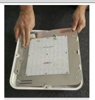
3. Push gear tray down opposite the swivel clips to take gear tray out.
