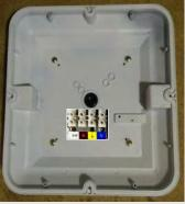
4. Mount base to the ceiling using 5mm x 25mm nail-ins. If IP65 rating is required use cable gland & side entry on the side opposite the LED driver.
