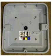
4. Mount base to the ceiling using 5mm x 25mm nail-ins. If IP65 rating is required use cable gland & side entry on the side opposite the LED driver.
